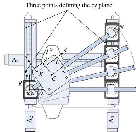
Fig. 9. Procedure for determining the base reference frame.
